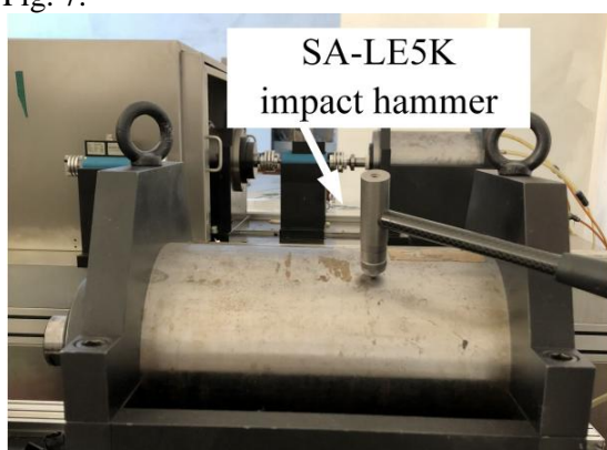
(a) Hammer test of natural frequency
