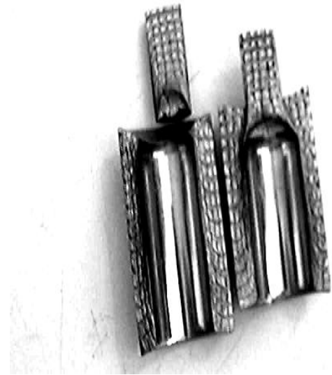
Fig. 5. Parts in lead obtained by combined extrusion with convex active plates: a-EC Pb 10x120 x20x30(2/2); b-EC Pb 10x105 x20x30(2/2).
