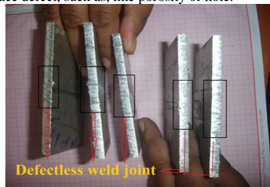
Fig 11 Cross-sectional image of Friction stir welded sample
