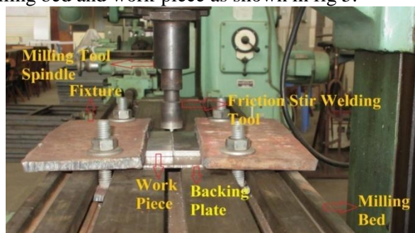
Fig 5 FSW experimental set-up
