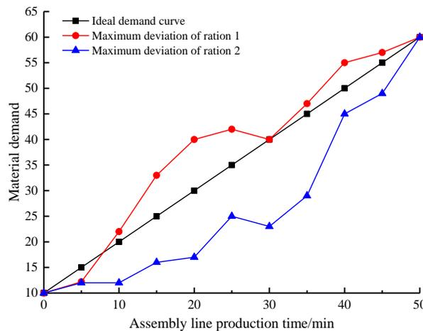
**Fig. 5 Comparison of material rationing demand curve in production workshop**
