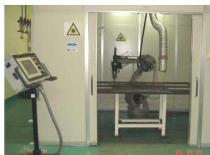
**Fig. 3 Nd:Yag laser machine equipment**
