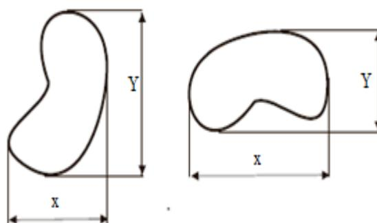
Fig. 3 Illustration of horizontal and vertical Feret diameters of a particle,  $F_x$  and  $F_y$ , respectively
