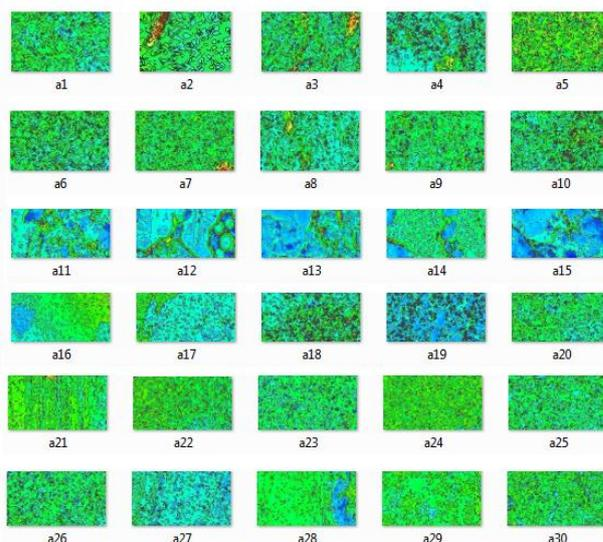
Fig. 6 Feret of microstructure of robot laser hardened specimens with different parameters of robot laser cell for hardening
