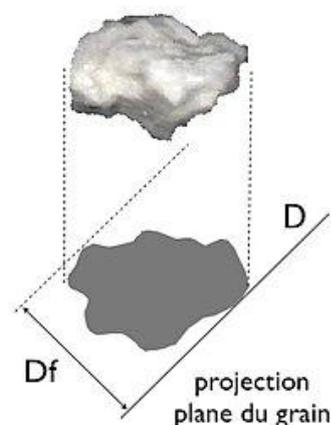
Fig. 4 Feret diameter applied to a projection of a 3D object
