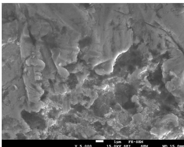
Fig. 1 Microstructure of SEM pictures of robot laser hardened specimens
