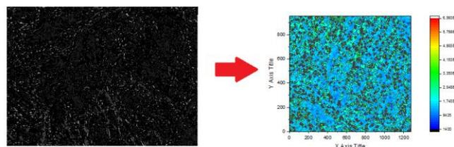
Fig. 2 Microstructure of robot laser hardened material (left), Feret from microstructure of robot laser hardened material (Right)
