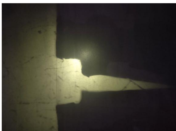
Fig. 3: NTOD Measurement using Profile Projector
