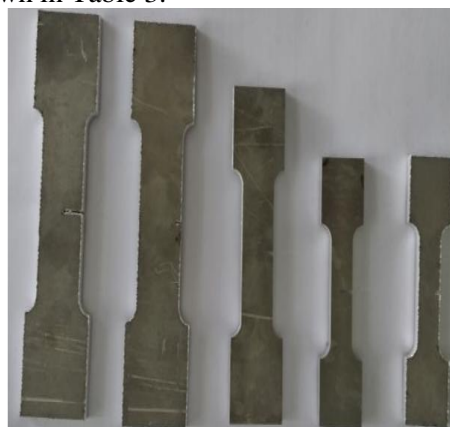
Fig. 1: Specimens as per ASTM E1820 standards
