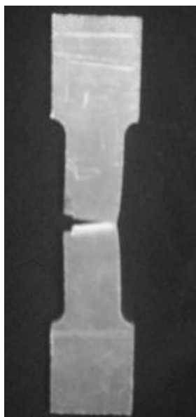
Fig. 2: Fractured Specimens at the end of load test
