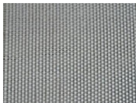
Fig. 2 Bidirectional glass fabric 450 g/m 2
