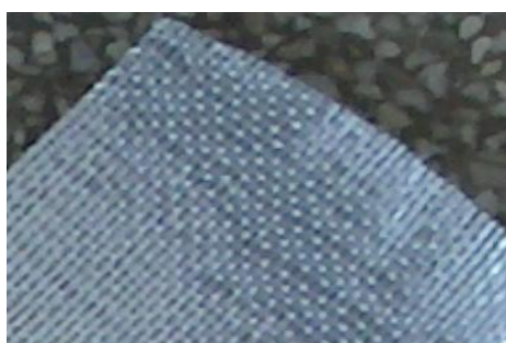
Fig. 1 Unidirectional glass fiber 225 g/m 2
