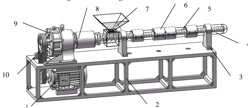
1.motor 2.frame 3.support frame 4.barrel 5.screw 6.electromagnetic heater 7.hopper 8.coupling 9.cycloid reducer 10.V belt drive
