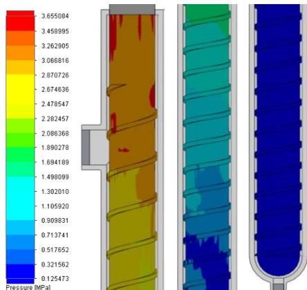
**Fig.15 Surface pressure distribution diagram of screw**
