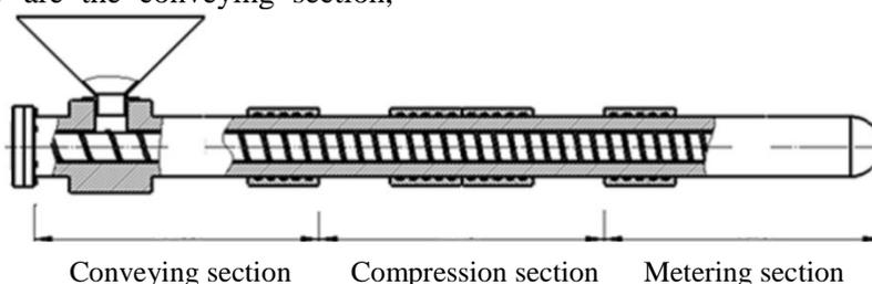
Fig.3 Segmentation of single screw extruder
