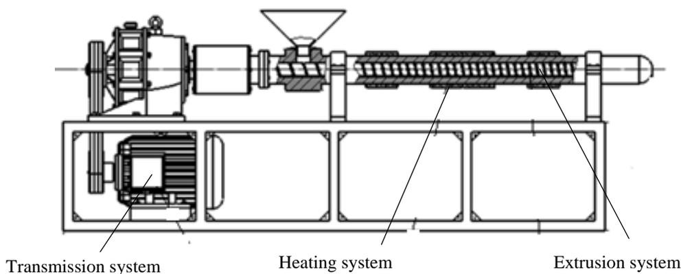
Fig.1 Plan view of single screw extruder
