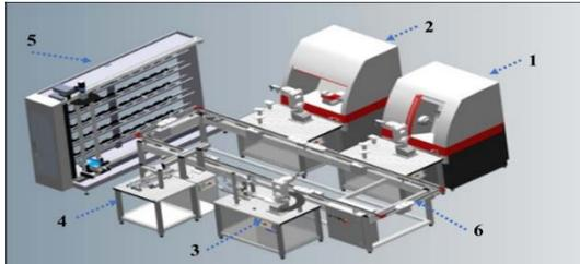
Fig. 1 3D Configuration of the iCIM 3000 system (Sobrinho & al, 2013).
