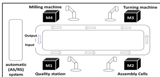
Fig. 2 The movement direction of parts in the iCIM 3000 system
