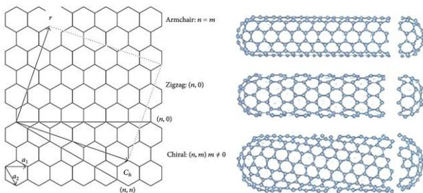
Fig. 3: Schematic representation of (a) formation of single-walled carbon nanotubes by rolling of a graphene sheet along lattice vectors which leads to the armchair, zigzag, and chiral tubes, and (b) the three types of carbon nanotubes [20].
