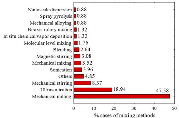
Fig. 7. Dispersion method involved in CNTs metallic matrix composites
