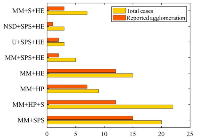
Fig. 11. Number of agglomeration cases with the fabrication method
