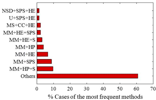
Fig. 9. Combination of CNTs dispersion method and consolidation method in CNTs-MMCs
