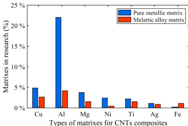
Fig. 6. Matrixes used in CNTs-MMCs research
