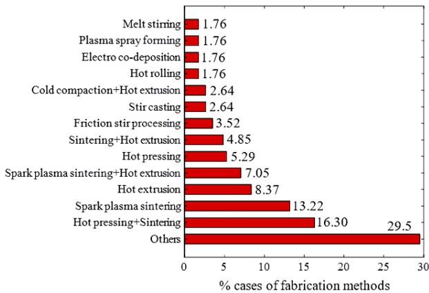
Fig. 8. Consolidation/Fabrication methods involved in CNTs-MMCs
