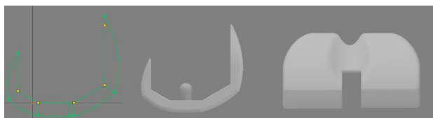
Fig. 8 Design stages of the custom femoral component
