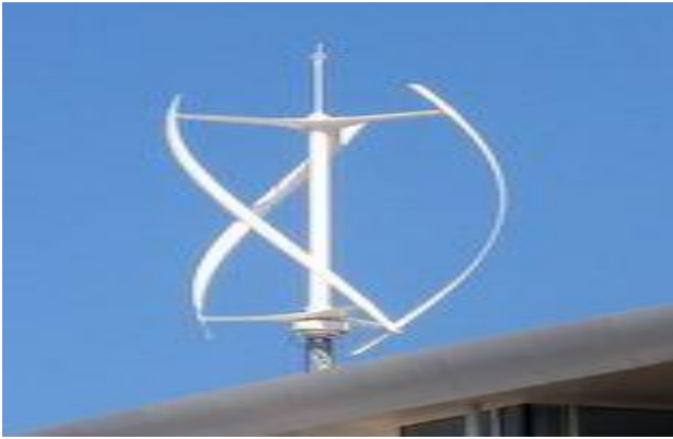
Fig .2 A vertical axis turbine rated at 6.5 kW
