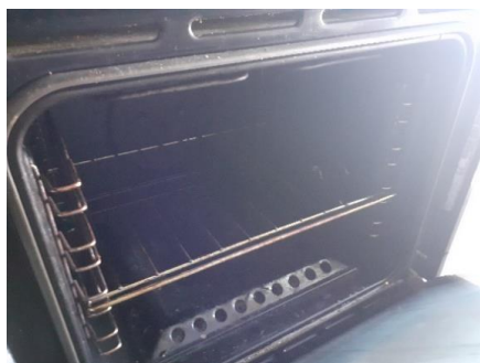
Fig. 1. 1.5 kW-laboratory electric heating oven of 60 L
