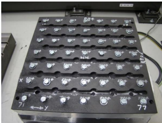
Fig. 3. State of the part after the trimming operation
