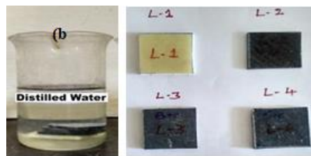
Fig. 2 (a) Hardness test specimens, (b) Test specimens under water absorption test.
