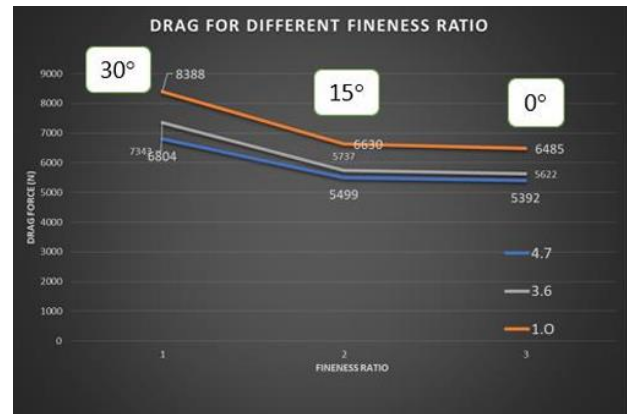
Fig. 8. Drag vs Different (1.0,3.6,4.7) Fineness ratio for 0^\circ, 15^\circ, 30^\circ Angle of Attack
